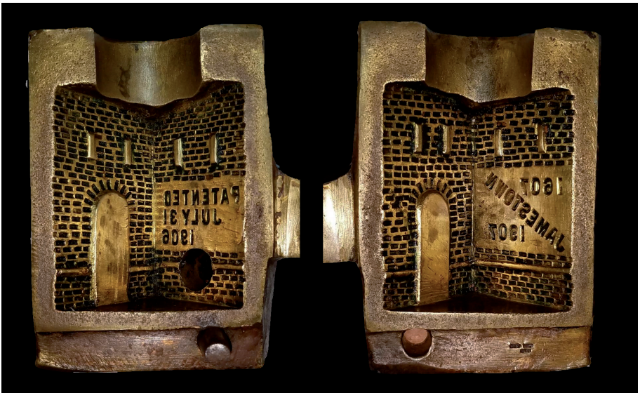
Figure 9: Bowl detail of the 1907 Jamestown Exposition pipe mould. Note the test of three brick shapes on the lower right hand corner of the pipe mould. Photograph by Paul Jung.
