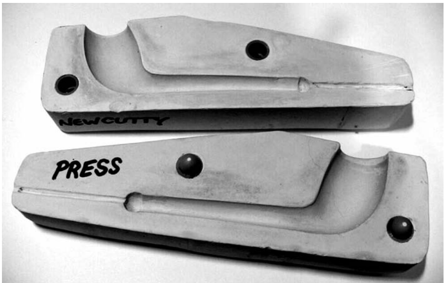
Figure 4: A plaster mould for press-moulding.
